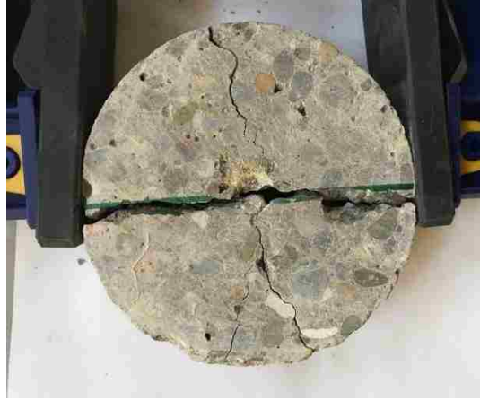
Figure 43: Minimum potential line with resultant fracture line
