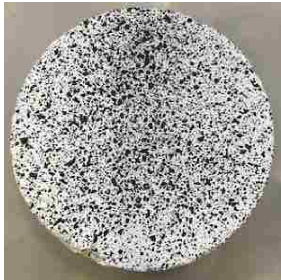
Figure 16: Specimen with stochastic pattern used for DIC
