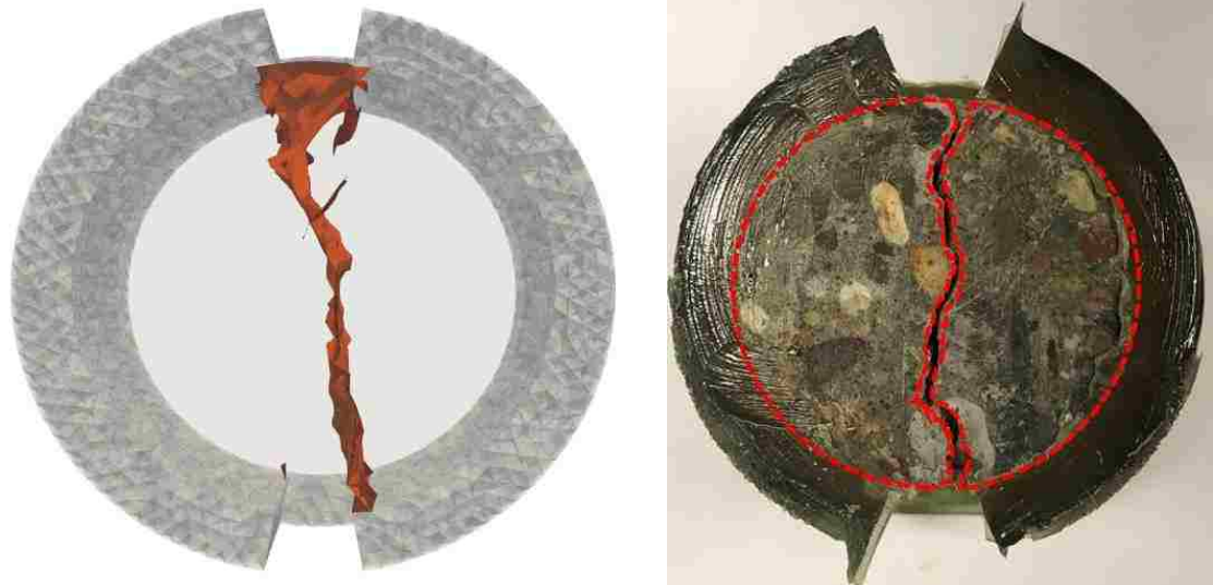
Figure 54: Validation of sleeved model fracture pattern
